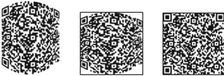
Fig. 2 Left: Bent QR code image. Middle: QRi_b . Right: QRi . Circumscribed rectangle of QRi_b formed in a square shape
