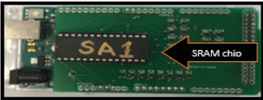
Fig. 9. SRAM PUF is developed by NAU cyber security Lab
